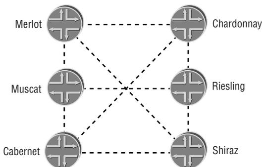
Each VC connection in the network appears as a point-to-point interface from the perspective of the router. In reality, however, the physical ATM connectivity may be quite different. Figure 11.4 shows this second set of connections.
